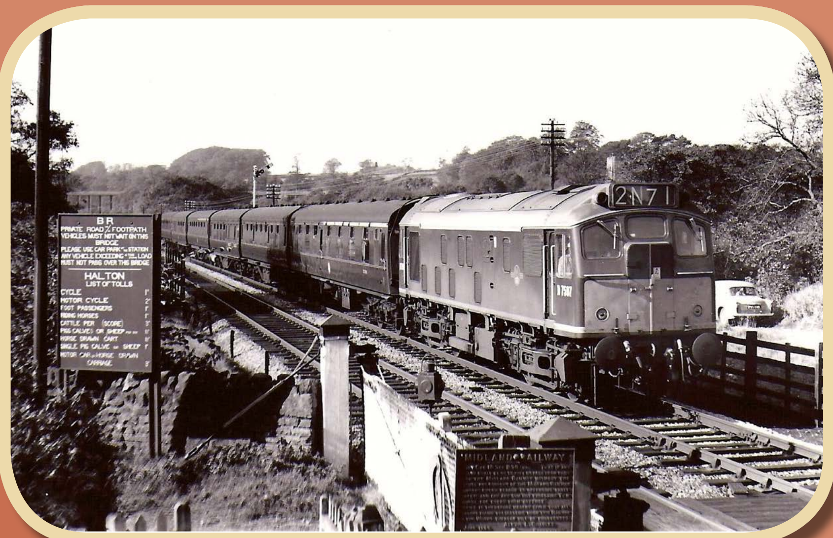
Class 25/2 diesel locomotive, D7587, approaching Halton with a Morecambe Promenade to Leeds service in the early 1960s. The restored list of tolls can be seen adjacent to the level crossing. The toll bridge over the River Lune is out of shot to the right. Courtesy John Robinson collection.
