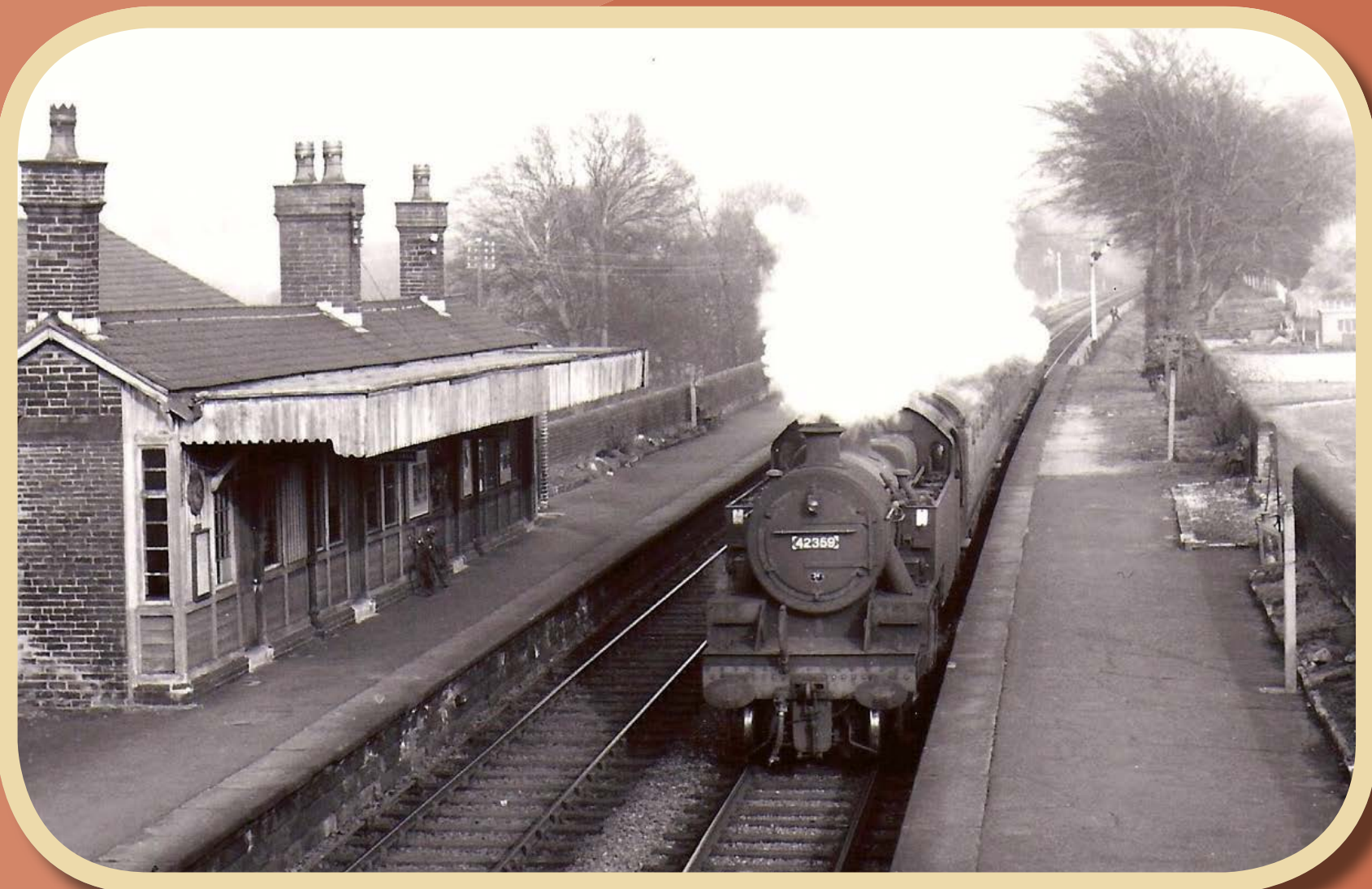
A late 1950s photograph of a westbound 3-coach stopping service to Morecambe Promenade, pulling into Halton, headed by a Fowler 2-6-4 tank locomotive, No. 42359. Courtesy John Robinson collection.
