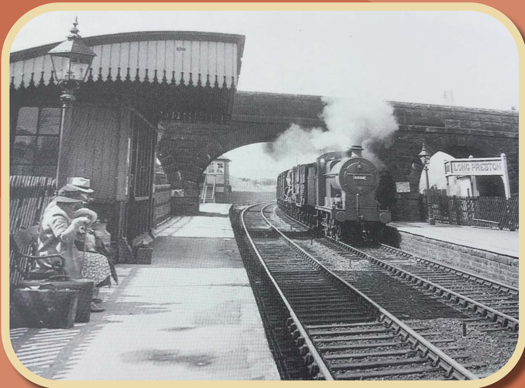
An LMS 4F 0-6-0 storms through Long Preston heading up freight as a family complete with suitcase await the next down passenger service in the late 1950s. Photo: D. Bins Collection
